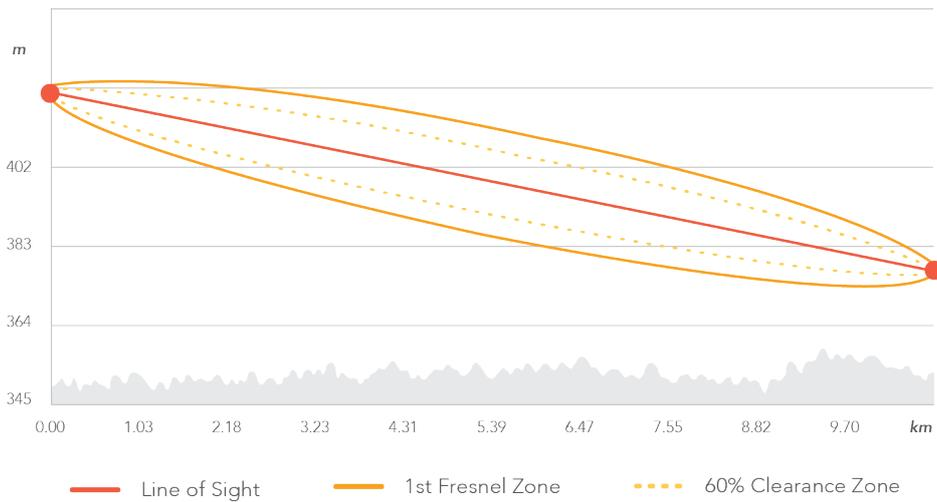
Link path profile showing a downward wireless link. It does not include buildings, but is otherwise with clear line of sight.
